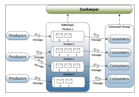
In the preceding diagram, a single node—single broker architecture is shown with a topic having four partitions. In terms of the components, the preceding diagram shows all the five components of the Kafka cluster: Zookeeper, Broker, Topic, Producer, and Consumer.
