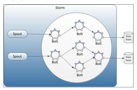
We can assume a Storm cluster to be a chain of bolt components, where each bolt performs some kind of transformation on the data streamed by the spout. Other than spout and bolts, a few other components are as follows:
