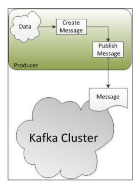
The producer connects to any of the alive nodes and requests metadata about the leaders for the partitions of a topic. This allows the producer to put the message directly to the lead broker for the partition.
