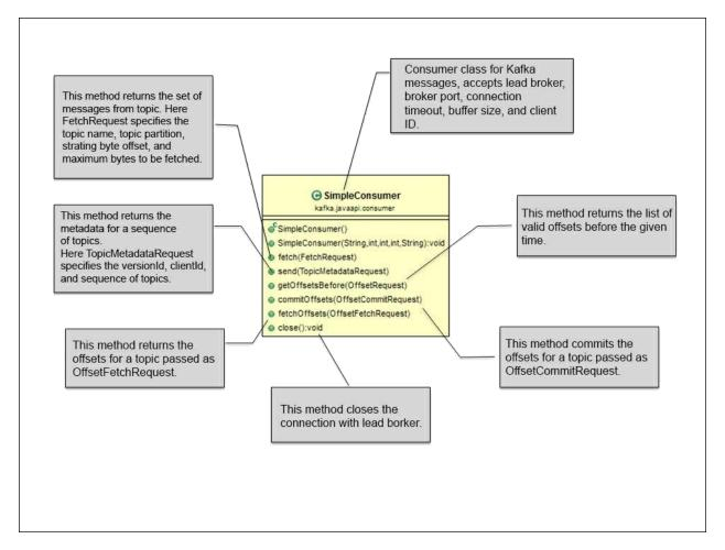
A simple consumer class provides a connection to the lead broker for fetching the messages from the topic and methods to get the topic metadata and the list of offsets.
